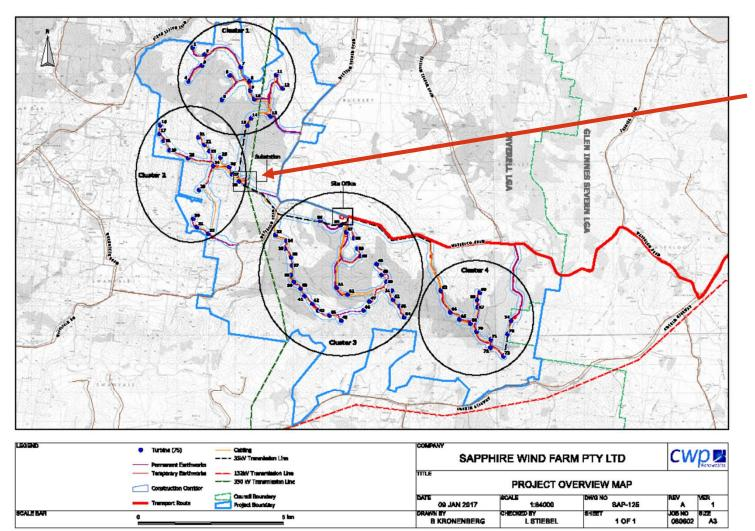
75 x 3.6 MW turbines in 4 clusters linking to new substation & into 330kv transmission line
